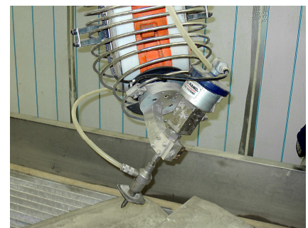
▲ Deform can perform three-dimensional cutting. Here are waterjet performed on Åkers plate.
